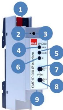
In addition to the normal programming button **3** the device allows activating the programming mode on the device front without opening the switchboard cover. The programming mode can be activated and deactivated via pressing simultaneously both buttons **7** and **8**.
