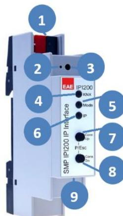
The Mode LED **5** can visualize the status of each KNXnet/IP tunneling connection.
