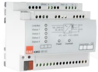
KNX Modbus Gateway
