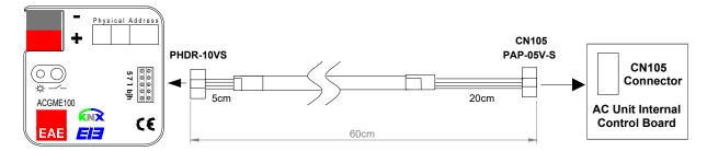
NOTE: Extending or shortening the connecting cable supplied with the device may cause it to malfunction. Keep the connection cable as far away from power cables and ground wire as possible.
