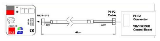
**NOT:** Extending or shortening the connection cable supplied with the device may cause it to malfunction. Keep the connection cable as far away from electrical wiring and ground wire as possible.
